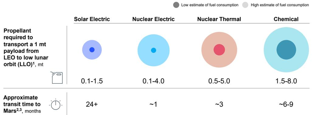
1. Entirety of spacecraft considered payload except for engine, power system, and propellant; assumes Isp of 1,000-10,000s for electric propulsion, 500-1,500s for nuclear thermal (NTP), and 250-450s for chemical and engine masses of 0.05-0.2 mt for solar electric (SEP), 0.7-2.0 mt for nuclear electric (NEP), 0.7-3.0 mt for NTP, and 0.1-1 mt for chemical; assumes full propellant mass is consumed by end of maneuver
